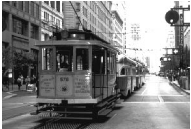
↑ Car #578 is the oldest operating electric in North America, 100 years old this year. This now fragile and rarely seen car survived long after her sisters as the system's sand car. This old timer was built new in San Francisco in 1895, was restored in the late 1950s and features purely mechanical hand operated brakes of the lever type as used today only on the cable car fleet.
