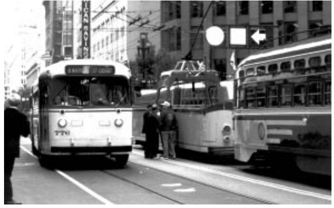
↑ Car #578 is the oldest operating electric in North America, 100 years old this year. This now fragile and rarely seen car survived long after her sisters as the system's sand car. This old timer was built new in San Francisco in 1895, was restored in the late 1950s and features purely mechanical hand operated brakes of the lever type as used today only on the cable car fleet.
